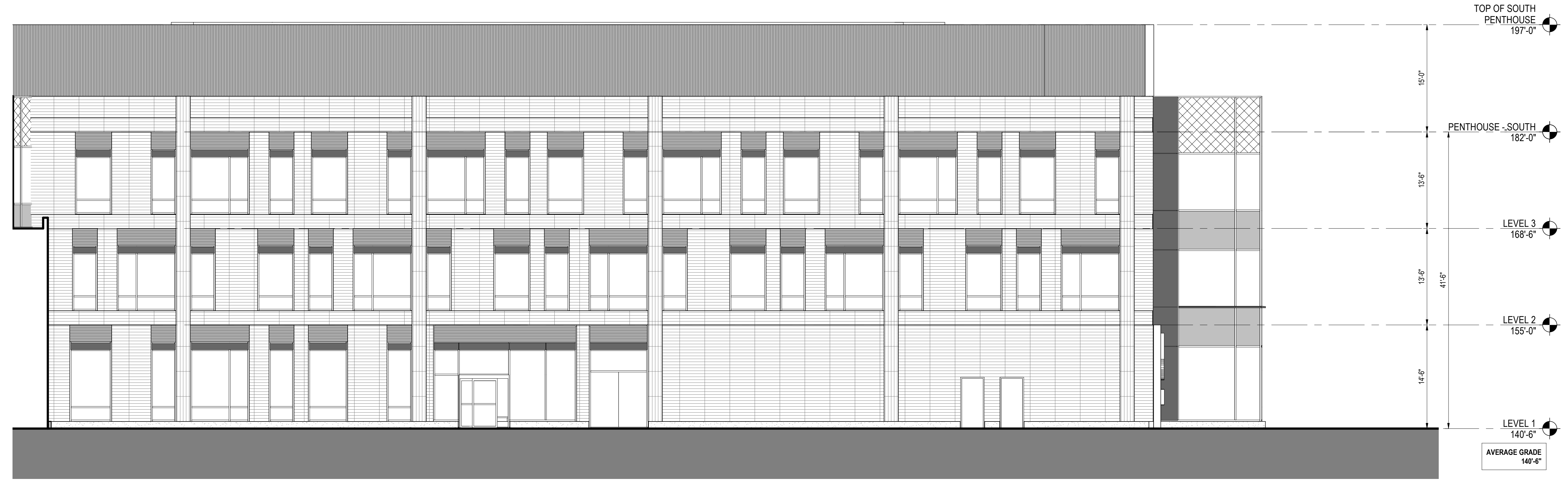
1 SOUTH BLDG - SOUTH ELEVATION LEVEL 1 - LOADING DOCK 1/8" = 1'-0"
